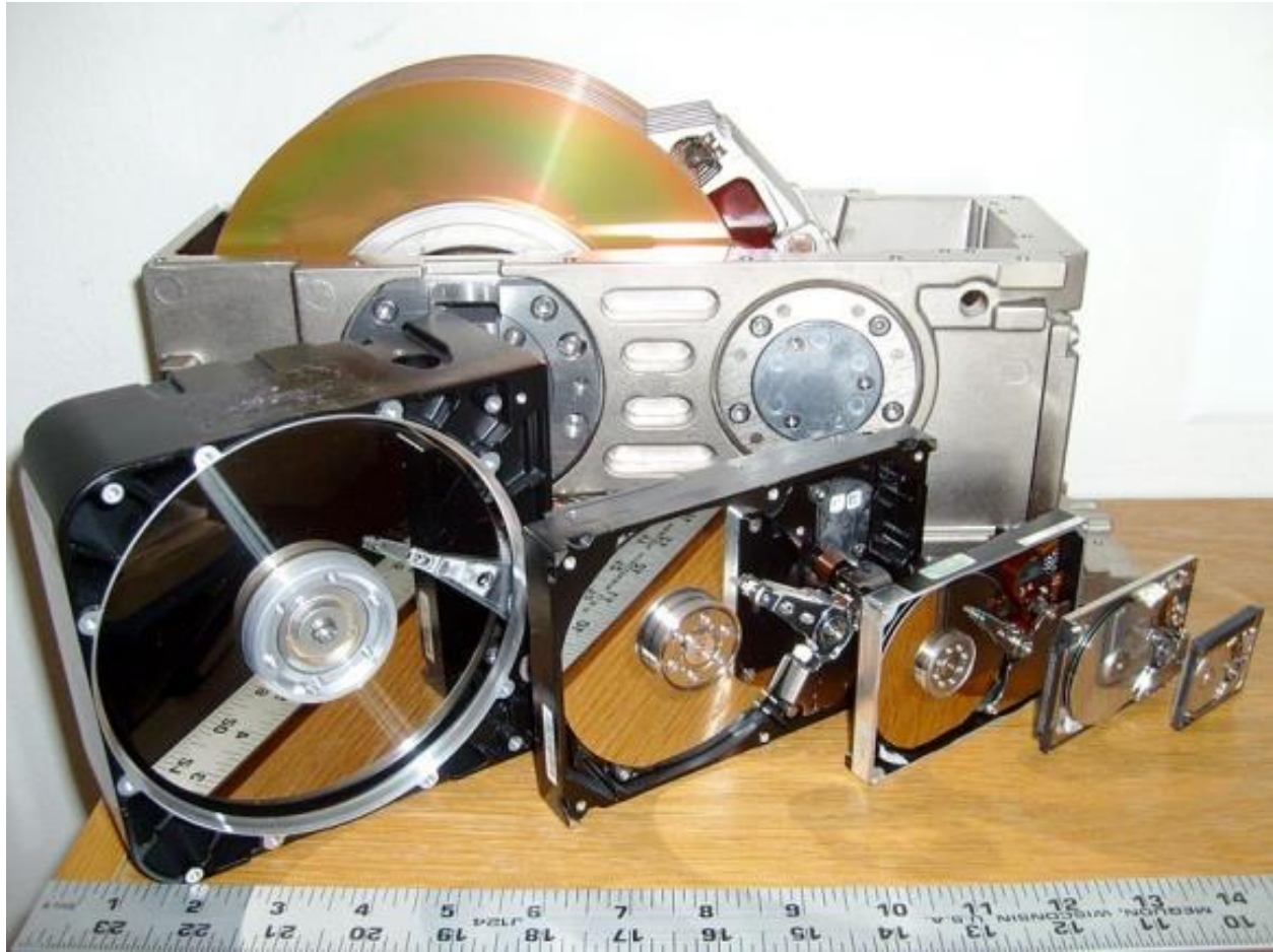
Three decades of disk drives, gradually shrinking to a more manageable size.
